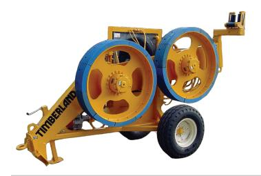
The PT40-1H/1DD is suitable for pulling or tensioning single conductor with infinitely variable tensioning control of the conductor.
